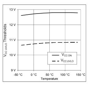
Fig. 2 - Under Voltage Lockout vs.
