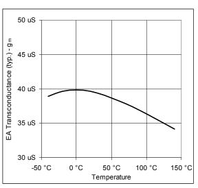
Fig. 6 - Voltage Error Amplifier Transconductance
