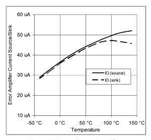
Fig.7 - Voltage Error Amplifier Source/Sink Current
