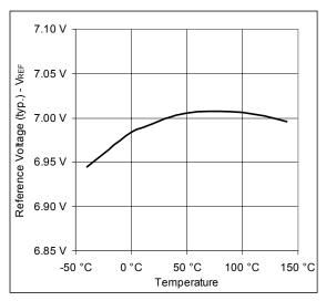
Fig. 5 - Reference Voltage
