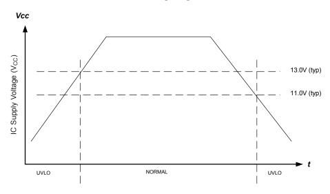
V<sub>cc</sub> Under Voltage Lockout
